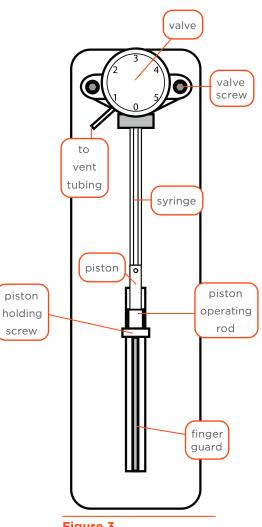
Figure 3 Syringe Installation
