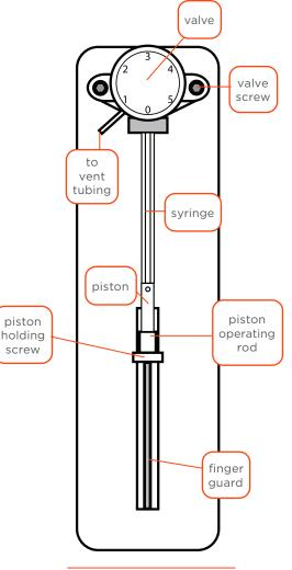
Figure 20 Syringe Installation
