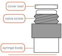
Figure 2 Cover Seal on Syringe
