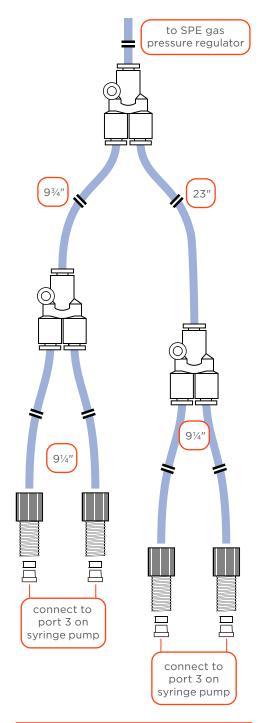
Figure 11 Air/Gas Supply Connections for ASPEC® 274 System
