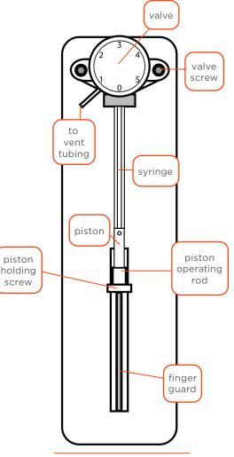
Figure 23 Syringe Installation
