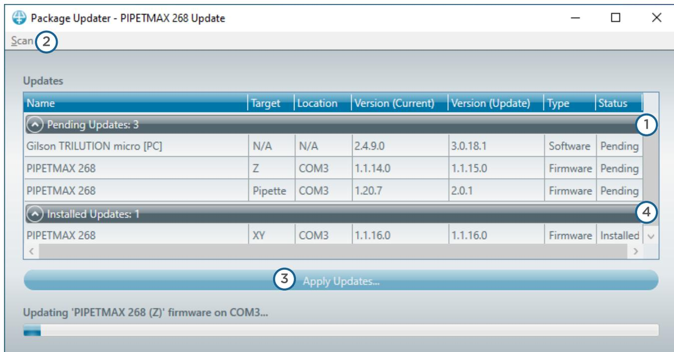
The Package Updater updates PIPETMAX software on the tablet or PC and firmware (if connected and necessary).
