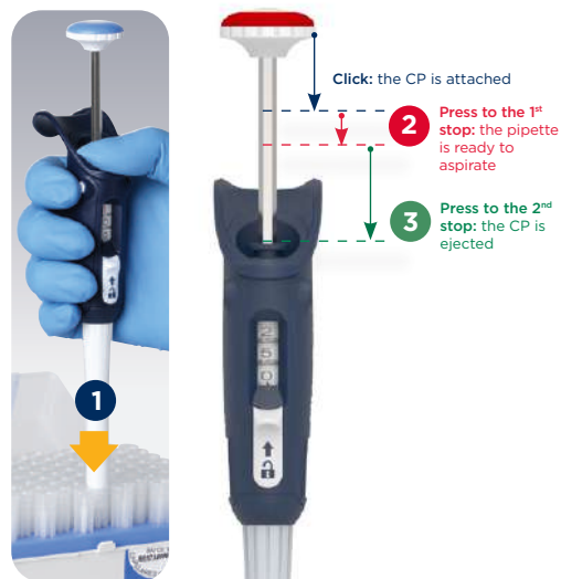
Figure 8 CP fitting on MICROMAN® E
